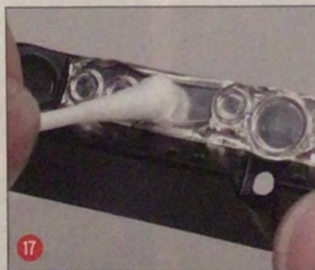
17 Instead of painting the instrument bezels, I decided to foil them. On a kit of this scale, I would have preferred separate, plated bezels. I use a cotton swab to ease the foil where I want it to go. After trimming the foil with a sharp knife, I was pretty happy with the results.
