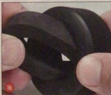
16 Each tire has a foam insert that needs to be installed. This was easy, and should keep the tires from collapsing over time.
