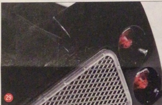
29 The little clip at the center of this photo is what holds the engine cover to the chassis. I had to open it ever so slightly, so it would snap onto the pins without breaking them off.
