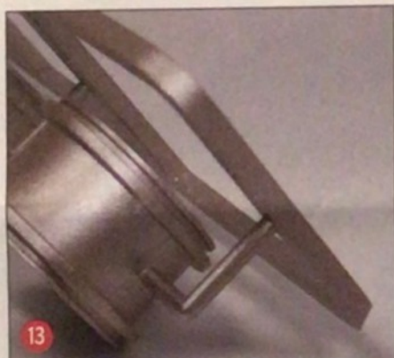
13 Trumpeter did go the extra mile by engineering the wheels to be attached to the sprue in the middle. This eliminates any chance of the wheel lip being damaged during removal from the sprue.
