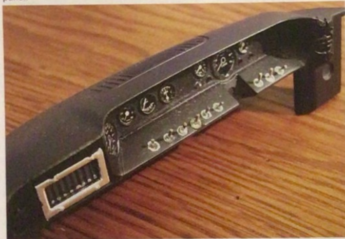
Below: I used sewing pins for the dash toggles and added wires to the fuse panel.
