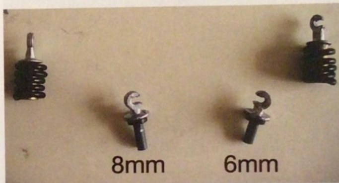
Test-fitting revealed that as built out of the box, the front suspension ride height is all wrong for a race car that ran 210 MPH—way too high. Not wanting a toy-like appearance for the model, I lowered it by nearly 3mm. To accomplish that, I first needed to shorten the assembled height of the springs. Ignoring the kit springs, I made my own from thin solder and compressed them tightly. I then shortened the inner shock rods by 2mm. Instead of being 8mm long, I made them 6mm. Then I joined the upper and lower shock halves with spring, being careful to orient the attachments for the control arms correctly—the upper faces inboard and the lower faces out.
